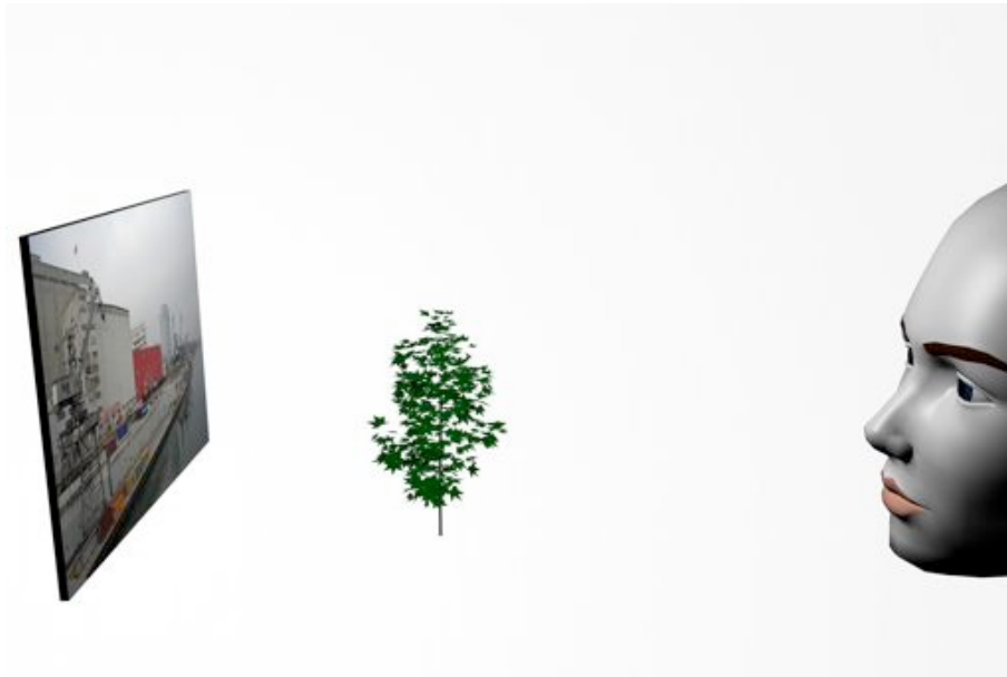
Fig 4. Conventional AR design uses a background screen and positions virtual elements in front of it.
